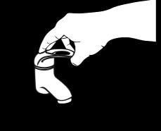
Step 2: Place your hand over the tap. The light sensor will recognise that your hand is there and fully turn on the device.
